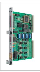
Equipped with DAQ PMUX firmware, Poller Mux cards form a dynamic front-end processor, collecting data from distributed RADC network controllers and relaying information to the central security system computer
